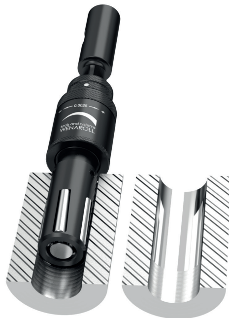
Left during Roller Burnishing / Right after Roller Burnishing
